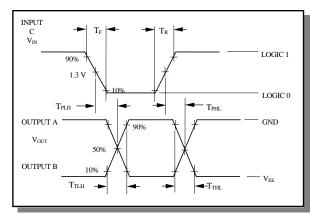
Note: See Switching Wave Forms for the definition of the switching terms. Supplies must be by-passed with .01  $\mu F$  Capacitors.
